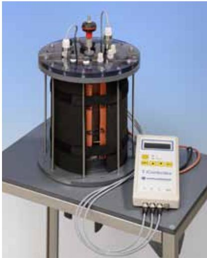
Figure 2: Reactor module incl. heating controller and stirrer
