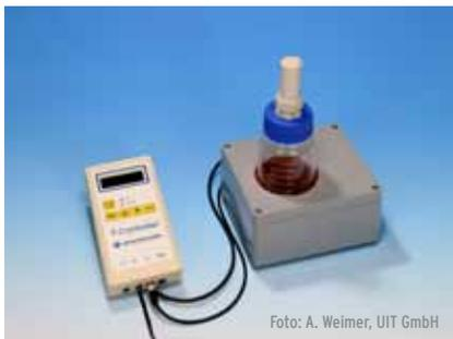
Figure 3: Test-set for identification of frothing of substrates
