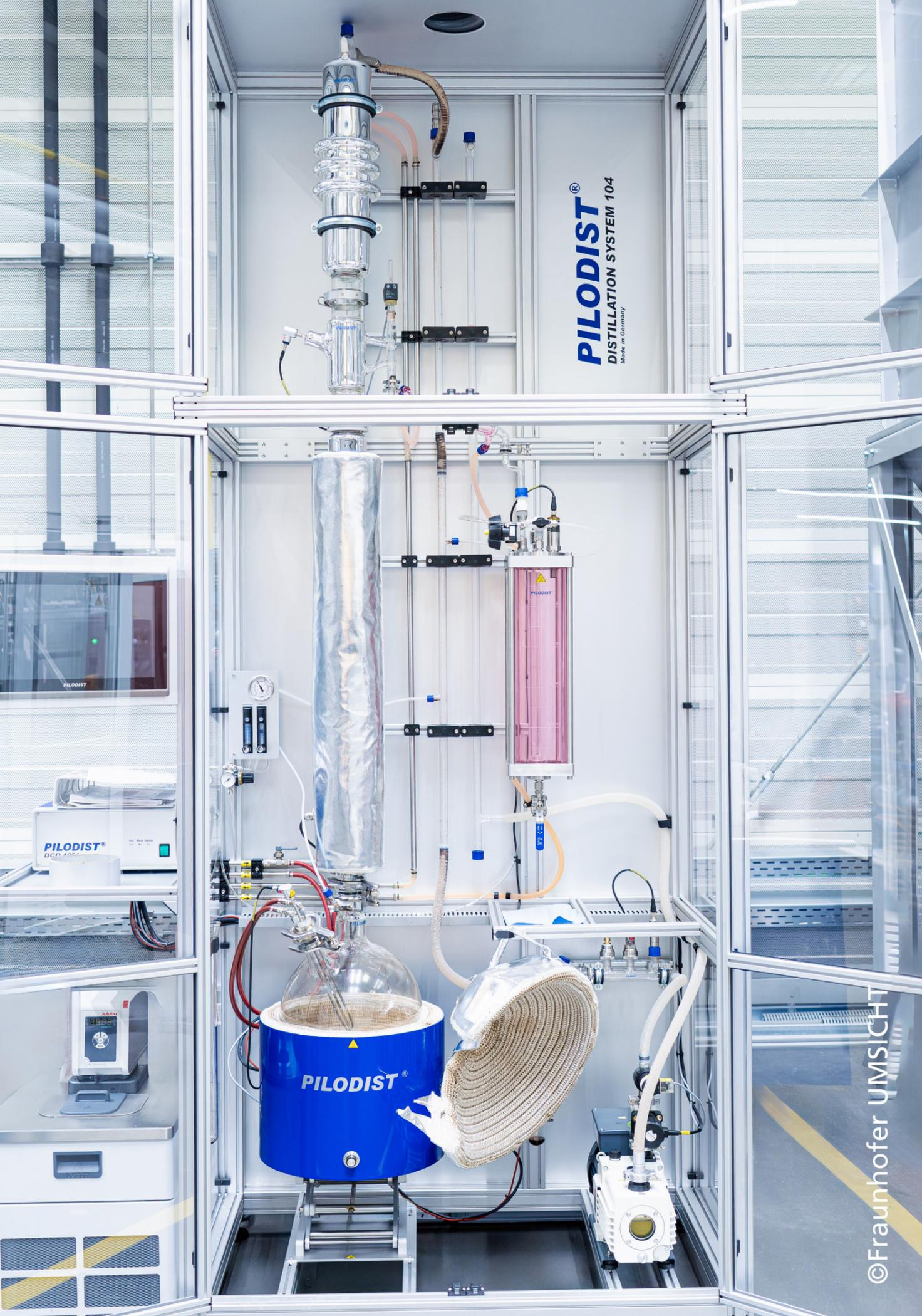
Abb. 6: 20 Liter Batch-Destillation am Fraunhofer UMSICHT
