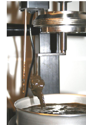
Figure 5.5-8: Adherence of solids to the surface of the ball (Source: BREHMER)
