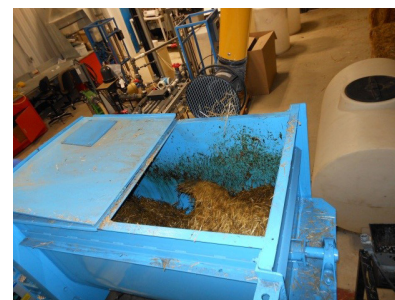
Figure 8.7-5: Paddle mixer used to prepare substrate mixtures for dry digestion (Source: InnoTech)
