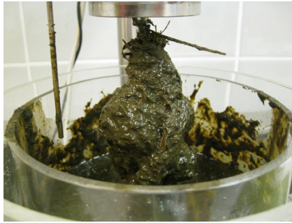
Figure 5.5-6: Wrapping of the vane shaft with long fibre substrate components (Source: BREHMER)
