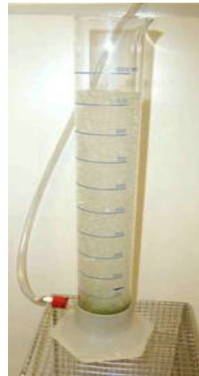
Figure 5.3-1: Foam generator with model foam (Source: UFZ)
