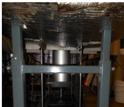
Figure 8.7-3: Pneumatic piston beneath dry digester and grating pulled down onto material to simulate pressure from material height inside the bunker (Source: InnoTech)
