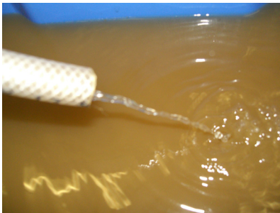
Figure 5.9-2: Overflow in the case of completed wet screening (Source: SCHNEIDER 2010)
