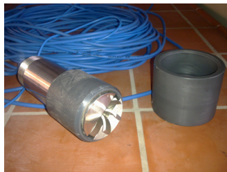
Figure 5.6-1: Sensor head of the vane anemometer for the measurement of the velocity in industrial scale biogas plants; built by Fraunhofer UMSICHT (Source: TU Berlin)
