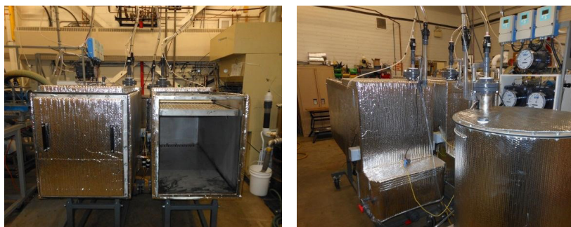
Figure 8.7-1: Dry batch digestion pilot plant at AITF. The pictures show the front of the system (left) and back (right) with a round percolation digester in the back (Source: InnoTech)
