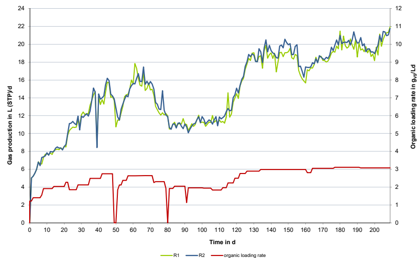
Figure 6.4-4: Gas production and organic loading rate of two continuous fermentation tests in parallel test (Source: DBFZ)
