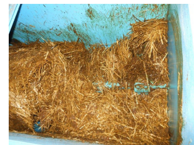
Figure 8.7-5: Paddle mixer used to prepare substrate mixtures for dry digestion (Source: InnoTech)
