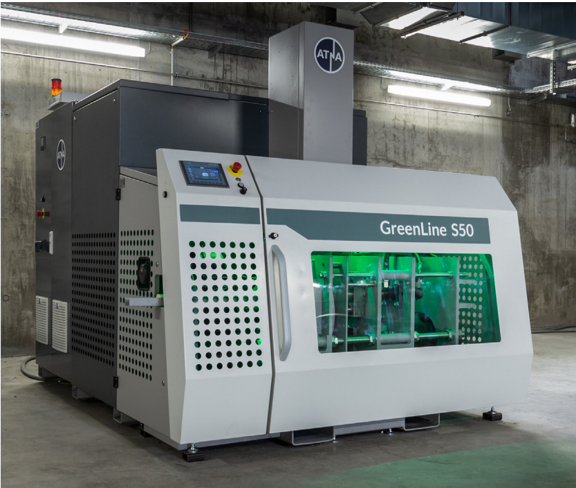
Abbildung 3 Brikettieranlage GreenLine S50 am DBFZ (© Wolfgang Grote / ATNA Industrial Solutions GmbH)
